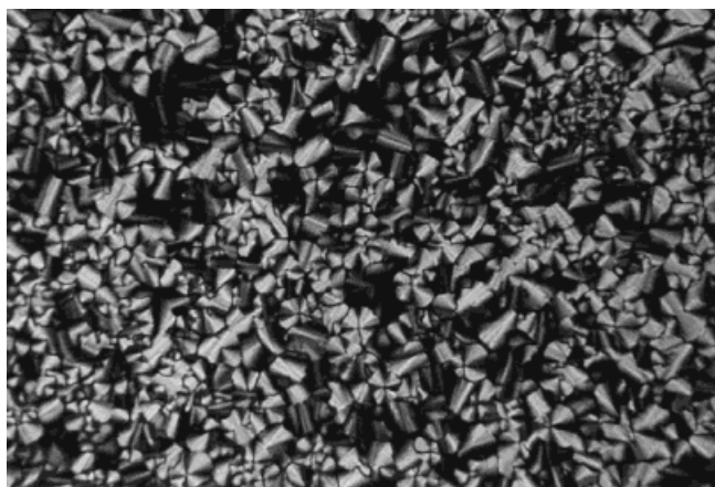
Figure 3. Texture of the columnar phase of [\text{CuSC}_{18}\text{H}_{37}] , on cooling from the isotropic liquid to 145^\circ\text{C} .
